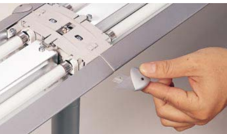
Locking segment design facilitates installation: Luminaire is deposited on support (no threading required) before triangular segment clip is fastened using tiny setscrew.
